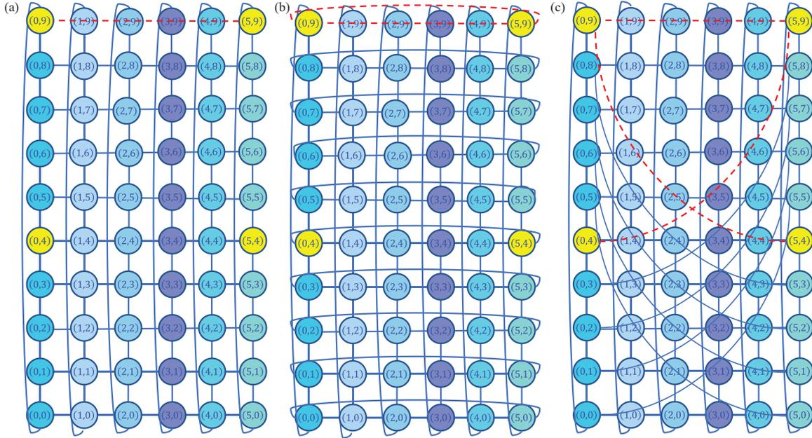
**Figure 7** (Color online) (a) The Mesh topology (with  $6 \times 10$  satellites); (b) the 2D-Tours topology (with  $6 \times 10$  satellites); (c) the Mobius topology (with  $6 \times 10$  satellites).
