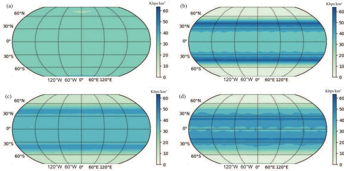
**Figure 6** (Color online) (a) The capacity coverage of single-layer polar orbit constellation (with 1440 satellites). (b) The capacity coverage of (b) single-layer, (c) two-layer, and (d) three-layer inclined orbit constellations.
