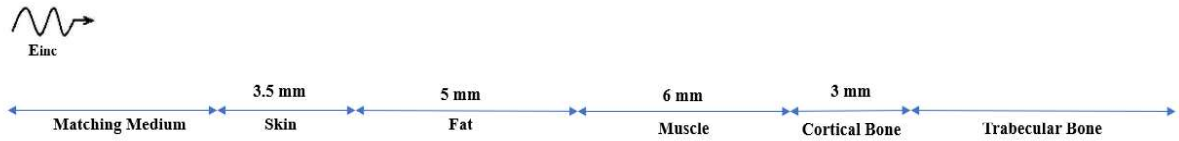
Fig. 2 The 1-D planar layered model of the human heel, which is composed of five layers: skin, fat, muscle, cortical bone, and trabecular bone. E_{inc} is the probing wave
