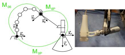
**Fig. 8** Ultrasound probe to robot base calibration principle.
