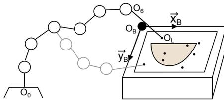
**Fig. 13** Geometrical model for x-ray image registration.
