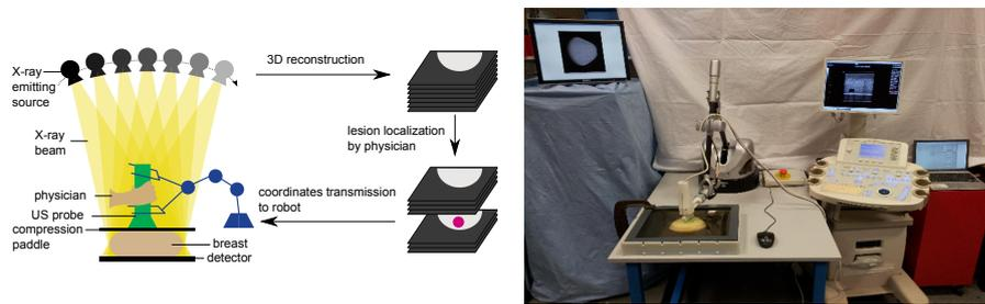
**Fig. 4** Novel system for robot assistance for combining US and DBT examinations. **Fig. 5** Test Setup
