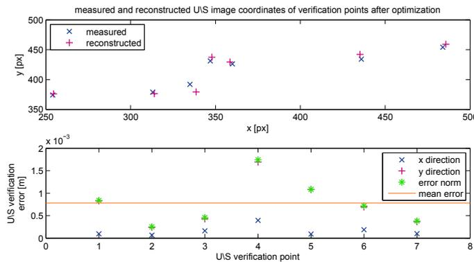
**Fig. 12** Parameter verification for ultrasound probe calibration.
