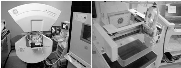
Fig. 3 Semi-automated US breast scanning system, [14].
