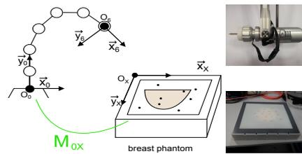
**Fig. 9** x-ray image to robot base registration principle.
