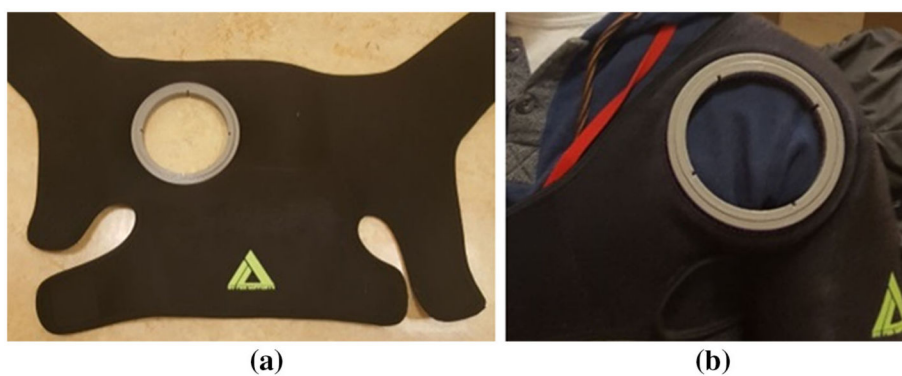
Fig. 5. New proposed mounting method is shown. a Ring adaptor is embedded in a shoulder brace, b shoulder brace with embedded ring adaptor on a volunteer's shoulder
