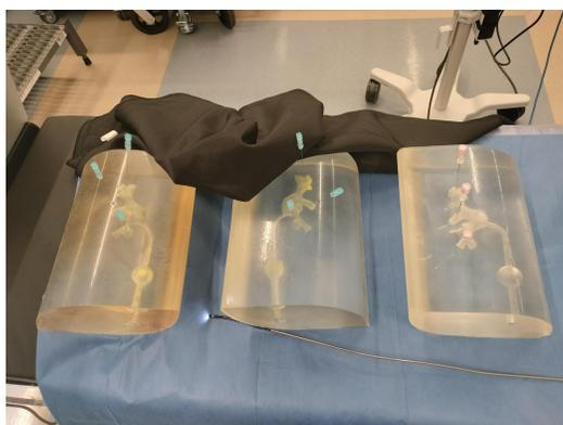
(a) Three kidney phantoms with needles inserted to simulate kidney stones. The needle tips are colored to prevent identification of the same fiducial.
