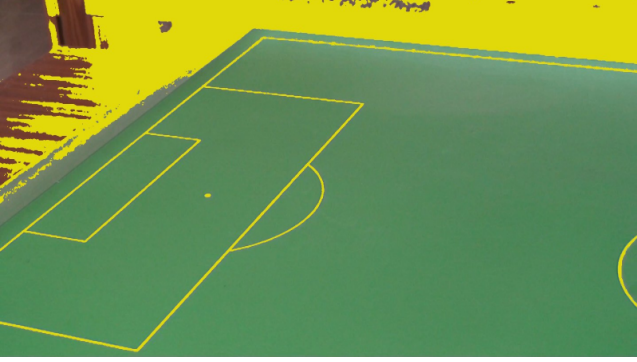
Fig. 6 Scale model image segmented by means of the CART method. The points classified as primitive are painted in yellow.
