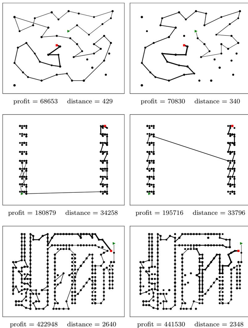
Fig. 3: The graphical representation of the solutions found by ACO (left) and ACO++ (right) for instances *eil51-10-bsc-01-03* (top), *pr107-05-usw-10-02* (middle), and *a280-10-unc-01-03* (bottom). The initial and final cities are highlighted using a green triangle and a red square, respectively. The lines connecting pairs of cities represent the route traveled by the thief, with the increasing line thickness corresponding to the thief's knapsack weight.
