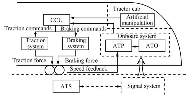
Fig. 1 ATC system scheme
