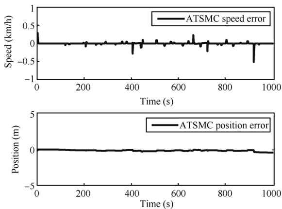
Fig. 7 Tracking error using adaptive terminal sliding mode control
