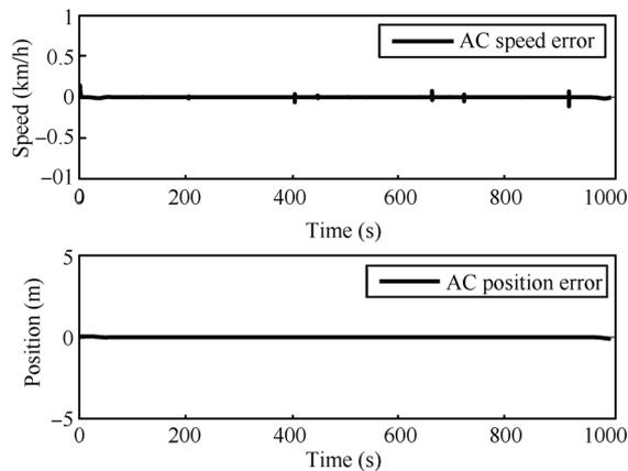
Fig. 6 Tracking error using adaptive control
