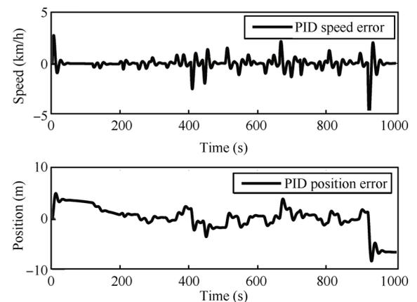
Fig. 5 Tracking error using PID
