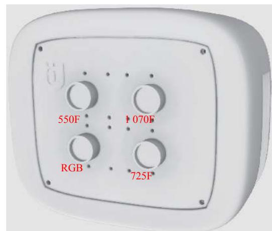
Fig. 2 Developed low-cost multispectral camera
