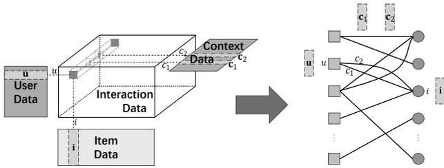
**Fig. 1** The data used for building a CARS. The mixture data of interaction tensor and user/item/context feature matrices are converted to an attributed user-item bipartite graph without loss of fidelity.
