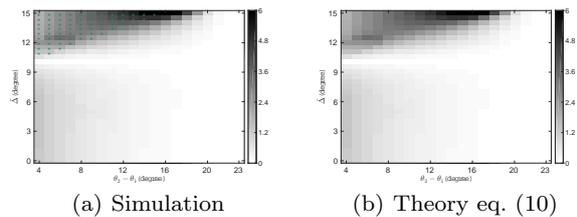
**Fig. 4**  $|E[\Delta\theta_1]|$  vs. the source angular separation  $|\theta_2 - \theta_1|$  and model angular dispersion  $\tilde{\Delta}$  (2 sources)
