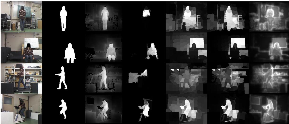
**Fig. 3** Saliency results of (a) sample images with (b) ground truth using models: (c) our GBPP-SbS (d) MDF [24] (e) MR [16] (f) RBD [20] (g) PCA [18]
