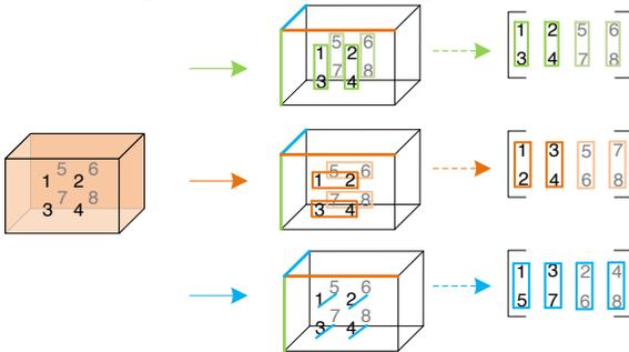
Fig. 1 Fiber unfolding of a three mode tensor.
