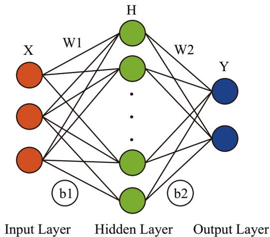
**Fig. 1** An example for the neural network with one hidden layer
