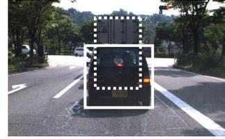
Figure 6. The case of two obstacles in front
