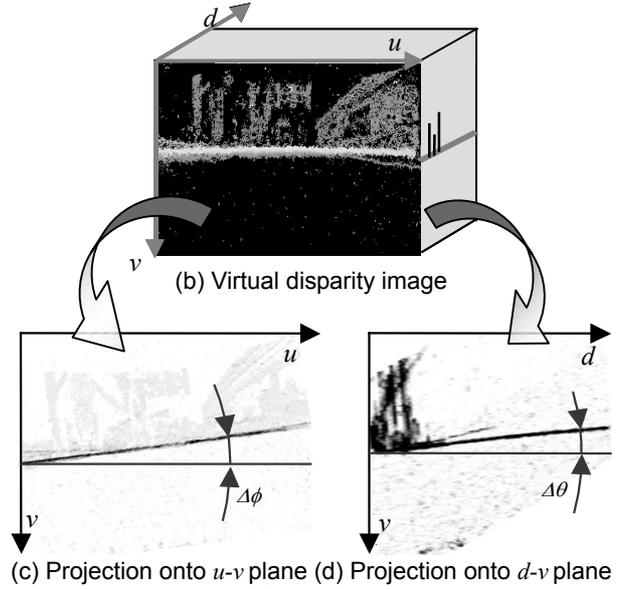
**Figure 4. Road surface extraction from virtual disparity image**
