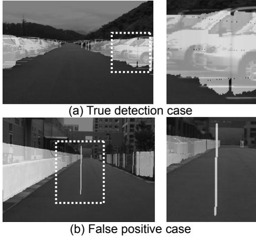
Figure 8. Obstacle detection results using raw data
