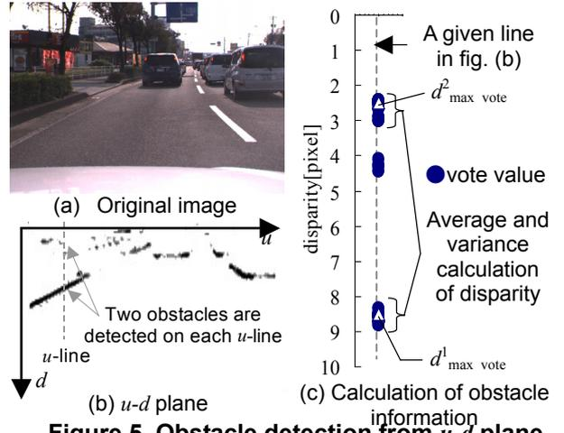
Figure 5. Obstacle detection from  $u$ - $d$  plane
