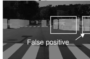
(b) Obstacle detection using OGM
