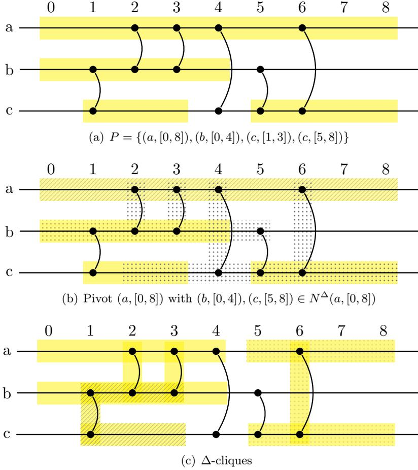
Figure 2: A exemplary set  $P$  of BRONKERBOSCHDELTAPIVOT, a possible pivot element (hatched) including its  $\Delta$ -neighborhood (dotted), and all maximal  $\Delta$ -cliques with respect to set  $P$ ,  $\Delta = 2$ .
