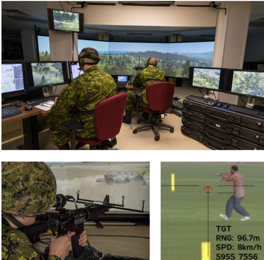
Fig. 1 Components of MT-ITS: VISS (top image), instrumented rifle (bottom left), and Smart Sight (bottom right). (Note: The bottom-right panel shows Smart Sight System aiming reticle with full target telemetry (range, speed, Military Grid Reference System location), shown as a vertical arrow and a calculated point-of-aim indicator to hit the target's center of mass shown as a red box.)
