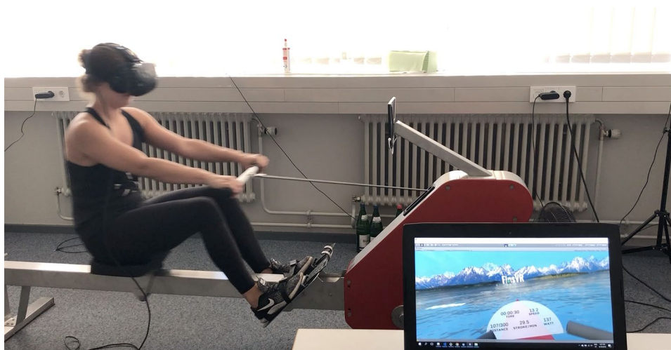
Fig. 1 Outside view on a setup for VR rowing exergame, where player is rowing with a HMD and VE is seen on the notebook screen
