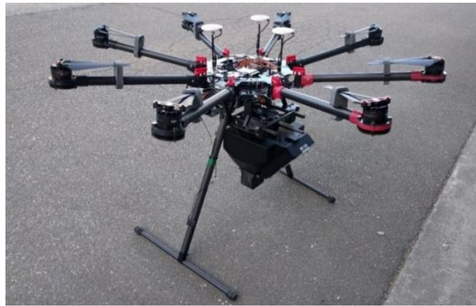
Fig. 2. The DJI S1000+ octocopter used in our experiments. The vermiculite dispenser, called “Bugbot” (see Fig. 4), was attached to the bottom of the UAV.
