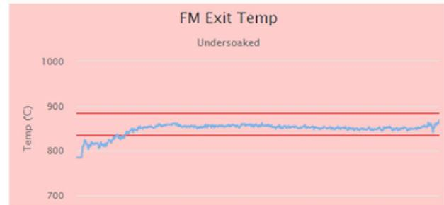
**Fig. 19** Example of a strip that has passed through the Finishing Mill subprocess that has been classified as having Width Pull and due to a combination of low temperatures and model error
