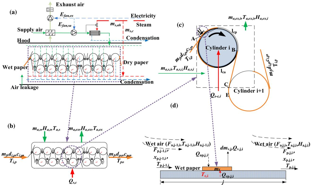
Fig. 3 Modeling of paper moisture evaporation in multi-cylinders dryer section
