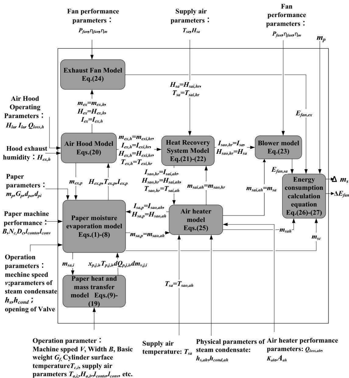
Fig. 7 Energy consumption model of drying system
