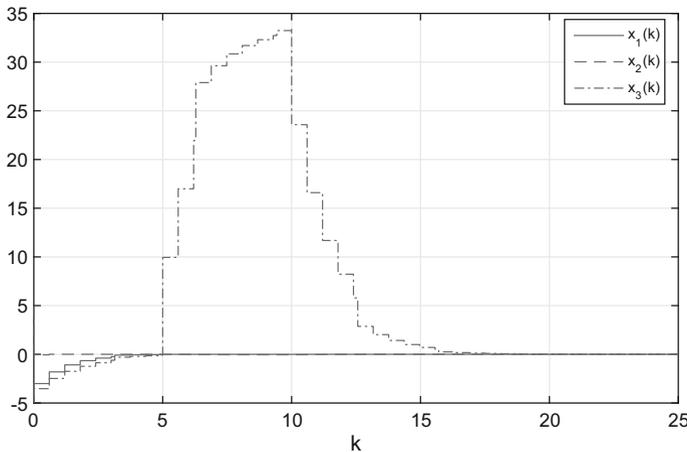
**Fig. 3** Evolution of the states with the controller in Table 2,  $d_M = 9$  (deviations from the desired values of  $M$ ,  $\theta$ , and  $\dot{\theta}$ )
