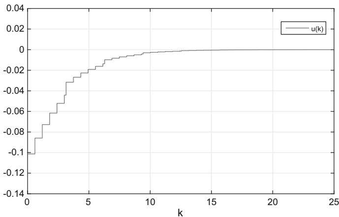
**Fig. 2** Evolution with the proposed controller of the control input (deviation from the nominal value of the actuator angle  $\theta_a$ )
