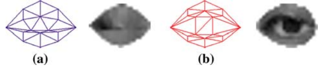
Fig. 3 Shape and appearance for the eyelid tracker (a). Shape and appearance for the iris tracker (b)
