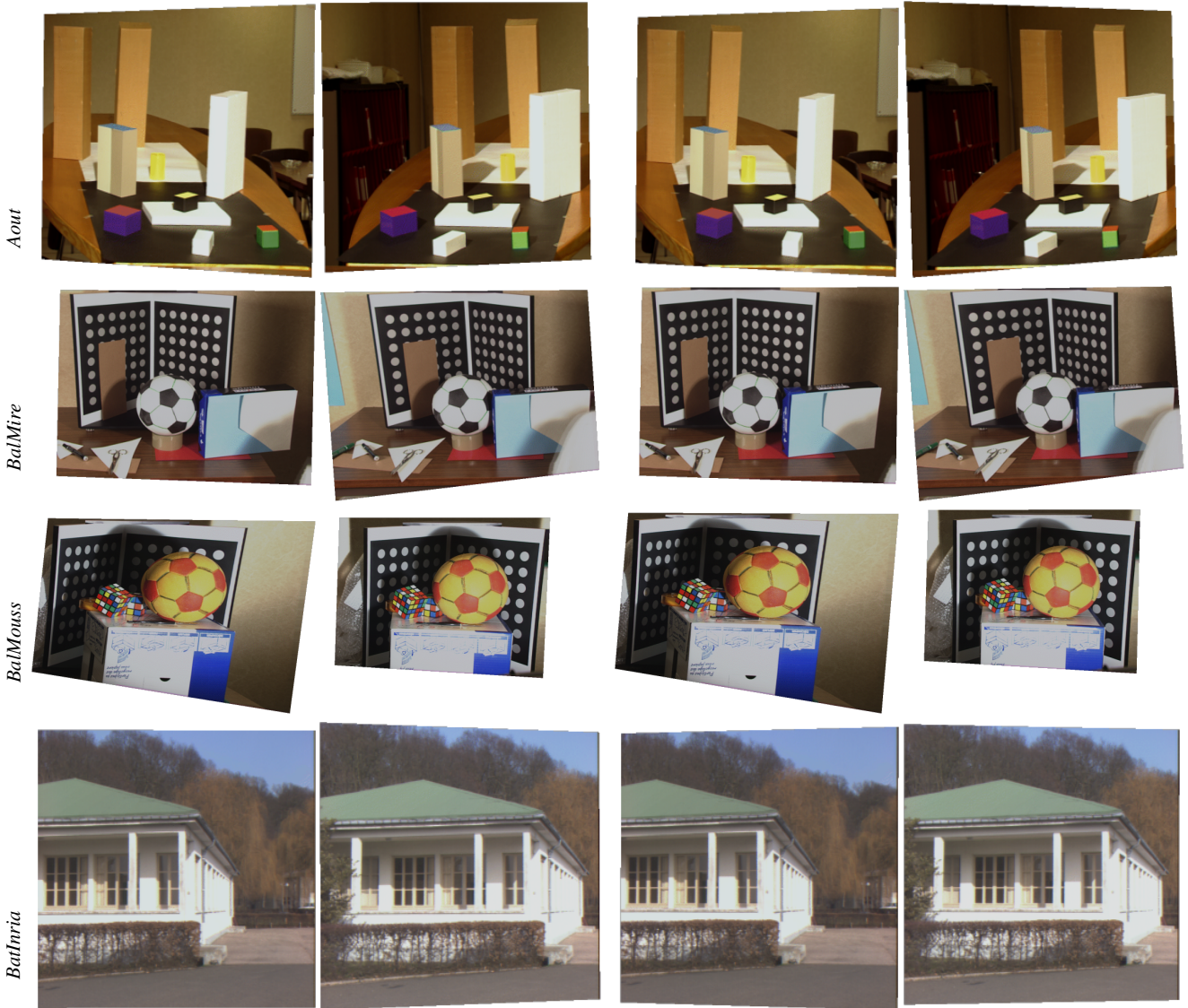
Fig. 1 Euclidean (left) and quasi-Euclidean rectification (right) of the SYNTIM pairs.
