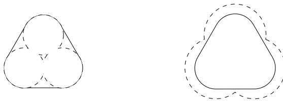
Figure 5: Left: the convex hull of a union of three balls. Right: By increasing the radii of the balls their union eventually covers the convex hull.
