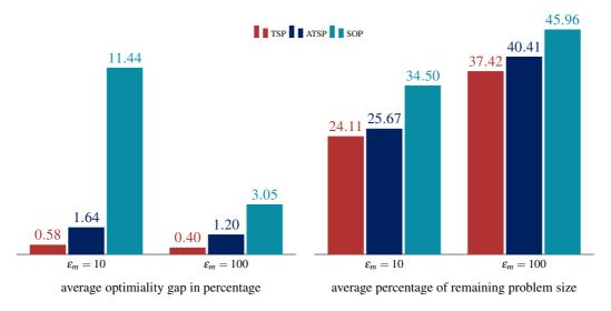
Figure 4: The average optimality gap generated by our MLPR model and the average percentage of remaining problem size after reduction when training our MLPR model on symmetric TSP instances and testing it on symmetric TSP, asymmetric TSP and SOP instances.
