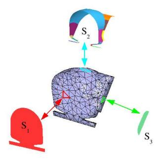
Fig. 3 The domain discretization is a piecewise decomposition of the domain; usually a mesh. Entities in the mesh (Vertices, Edge, Faces, and Regions) can be associated with entities in the geometric model. This association is referred to as "classification" of mesh entities on model entities. Reverse classification associates model entities with mesh entities residing on that portion of the model.
