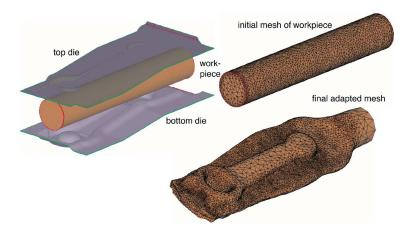
Fig. 6 Metal forming example.
