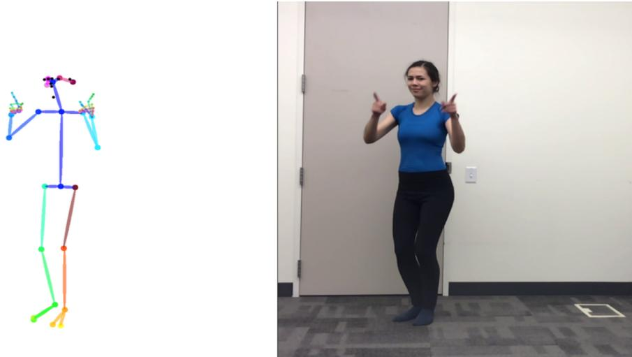
Figure 1: Pose detection illustration taken from (Chan et al., 2018). Skeleton points represent joints.
