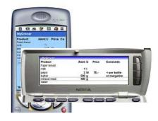
Figure 4. Access to retail m-services via cellular wireless mobile devices: user authentication (left) and shopping list editing (right) on wireless enabled personal digital assistant and cellular mobile telephone (both Java 2 Micro Edition capable).
