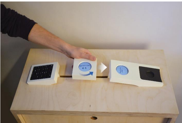
Fig. 6 Left: The vendor moves the traveller towards the customer module, the screen rotates accordingly. Right: The traveller resides at the customer module
