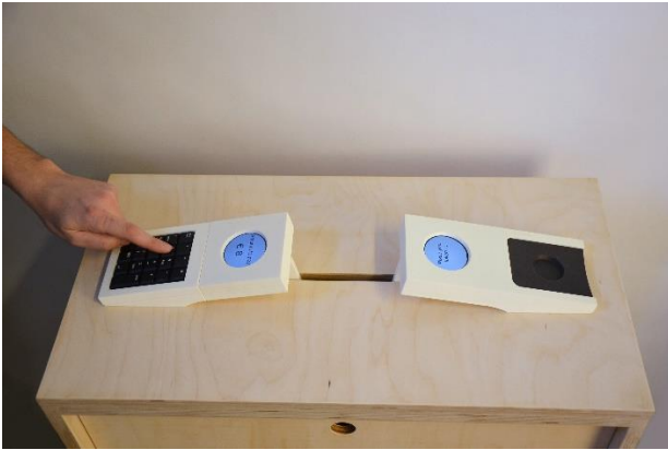
Fig. 5 The vendor enters the price on the keypad of the vendor module
