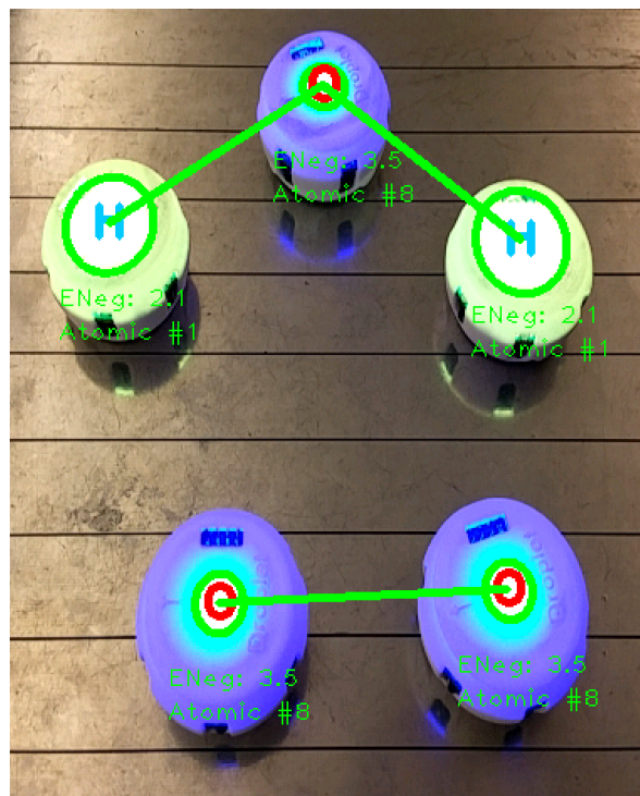
Fig. 1. Five droplets forming an O 2 and a H 2 O molecule. Augmented Reality on a smart phone is used to show the actual bonds, electronegativity and atomic number.
