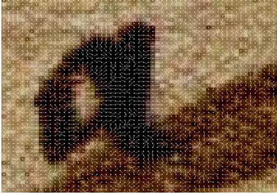
(a) Orientation of the gradient vectors in the case of the Perona-Malik process
