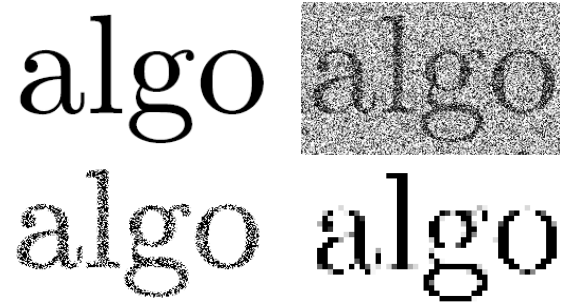
Fig. 19 Distortion in an extract of a document image; the original document image and its distorted versions.
