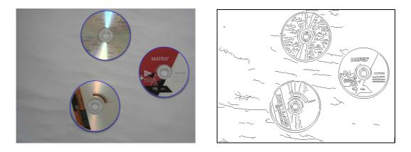
(a) (b) **Fig. 7.** Multiple circle detection on real-life images: (a) the original image holding the best three detected circular shapes, (b) the edge image after applying the Canny algorithm.
