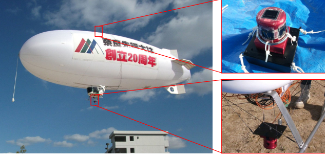
Fig. 3 Unmanned airship and omnidirectional cameras. Two cameras are mounted above and below the aircraft. ND filters are attached to the camera above. A GPS antenna is also mounted atop the aircraft.
