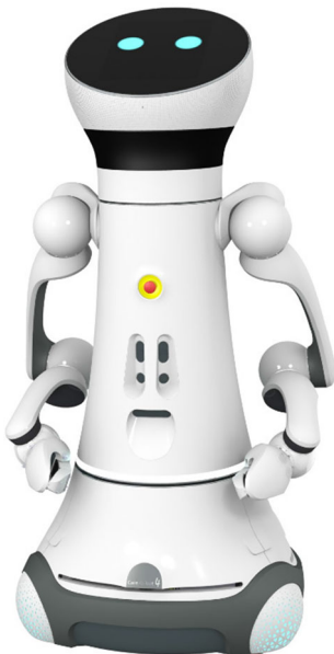
Fig. 5 Care-O-bot4 full robot. Developed by Mojin Robotics
