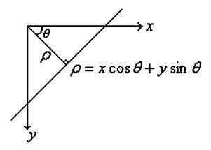
Fig 4. Representation of a straight line.
