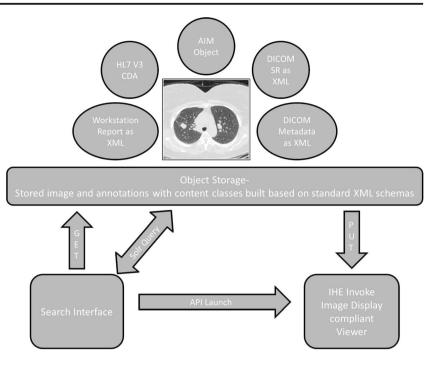
resulted in the path to a unique image file that met these parameters being returned through the API, which was then used in a batch file where a GET command brought that specific image locally over the Internet in a secure transaction. The image was subsequently launched using the IHE Invoke Image Display [6] profile and displayed for the user to visualize and interact with.
