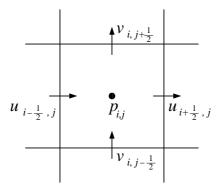
**Fig. 2** Staggered grid discretization in which the velocity field u = (u, v) and Eulerian body force  $f = (f_1, f_2)$  are approximated at the centers of the cell edges, and in which the pressure p is approximated at the cell centers.
