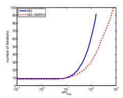
Fig. 3 Iteration counts for the multigrid solver and for multigrid-preconditioned GMRES to reduce the residual by a factor of  $10^{-6}$  as a function of the stiffness. The stiffness is scaled by the maximum stiffness from the explicit-time scheme,  $\alpha_{\text{exp}}$ .
