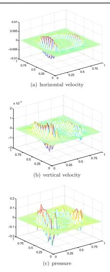
Fig. 5 Plots of the velocity and pressure corresponding to an eigenvector or the multigrid iteration matrix with eigenvalue 0.8522 for relative stiffness  $\alpha_{\rm exp}/\alpha$ .
