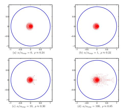
Fig. 4 Plots of the eigenvalues of the multigrid iteration matrix for four different values of the relative stiffnesses. The value of  $\rho$  is the largest eigenvalue excluding the trivial eigenvalue of 1.
