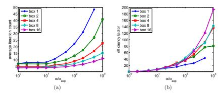
Fig. 9 (a) Average number of iterations of the MG-GMRES method per time step in the implicit-time simulation. (b) The efficiency factor is the expected speed-up gained by using the implicit method in place of an explicit method.
