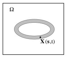
Fig. 1 The physical domain  $\Omega$  contains the immersed elastic structure. The position of each material point s at time t is given by  $X(s,t) \in \Omega$ .
