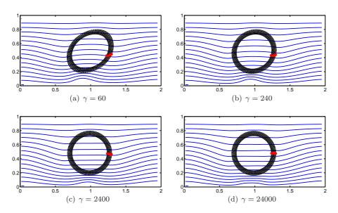
Fig. 8 Streamlines and structure location at time t=1 for a range of stiffnesses. The red markers on the structure are used to highlight rotation and internal deformation. At the beginning of the simulation the red markers were aligned horizontally in the x-direction.
