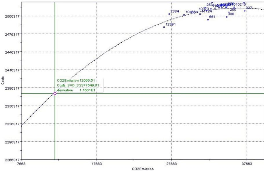
**Fig. 4** Pareto optimal frontier for selected results in Phase-I
