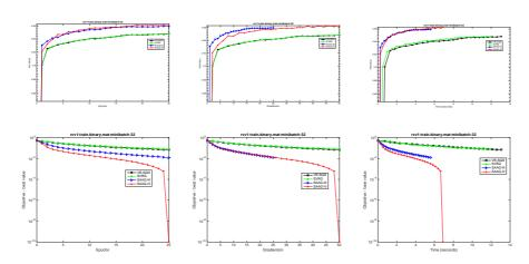
Fig. 4: Comparison of SAAG-III, IV, SVRG and VR-SGD on non-smooth problem using rcv1 dataset with mini-batch of 32 data points. First row compares accuracy against epochs, gradients/n and time, and second row compares suboptimality against epochs, gradients/n and time.
