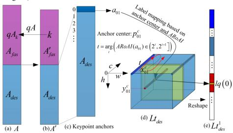
Fig. 3. Illustration of the mapping from anchor to tensor. (a) Array of all the anchors A. (b) Array of all the anchors inside image A'. (c) The list of keypoint anchors. (d) 3-D label tensor  $Lt_{des}$ . (e) 1-D label tensor  $Lt_{des}^1$ .
