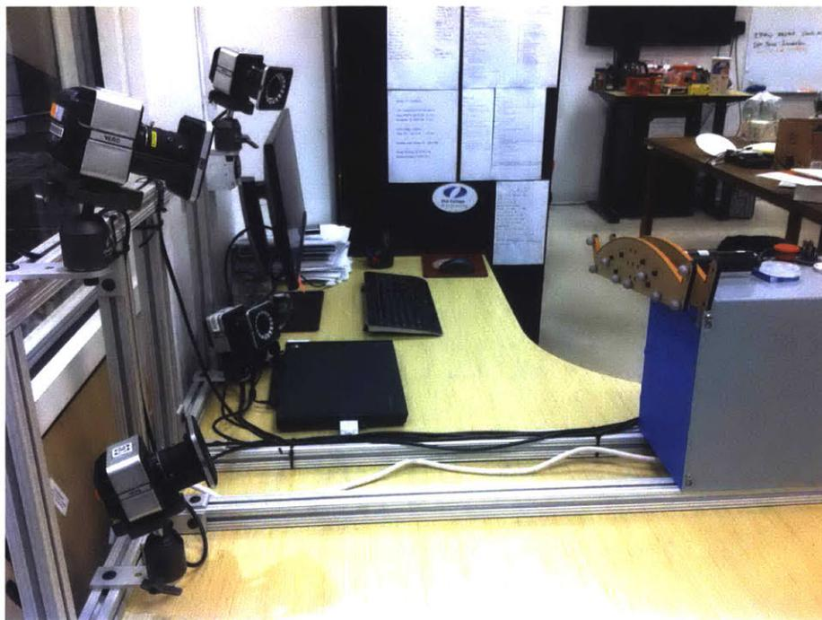
Figure A-2: A picture of the experimental setup. The hand, control box, and motion capture cameras can all be seen.
