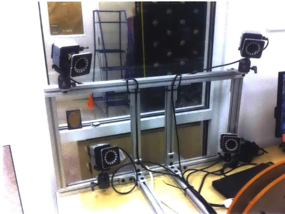
Figure A-3: The cameras used for the motion capture system.
