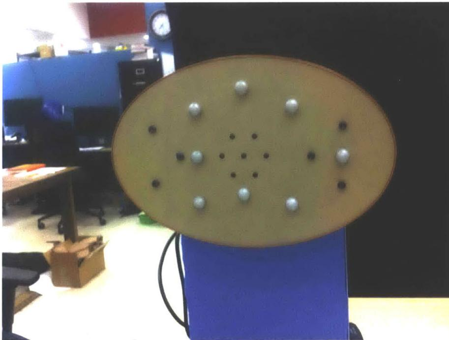
Figure A-5: IR reflective markers are attached to the hand, allowing the motion capture system to measure its position and orientation.
