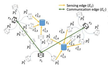
**Fig. 1** Description of multi-robot task allocation for multi-target tracking. In this example, three robots  $(\mathbf{r}_1, \mathbf{r}_2, \mathbf{r}_3)$  are tracking two moving targets  $(\mathbf{t}_1, \mathbf{t}_2)$ . Each robot has five motion primitives  $(\mathbf{p}_m^i)$  to choose from at each time step. c represents the cost of observing a target from a motion primitive.
