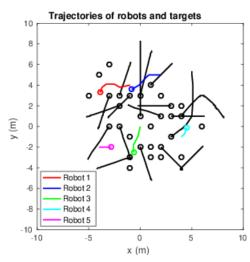
Fig. 15 Plot of trajectories of robots and targets applying the local algorithm to the simulation given in Figure 14. Black lines represent trajectories of thirty targets.  $\circ$  denotes the end position of trajectories. The algorithm was performed for 40 seconds.
