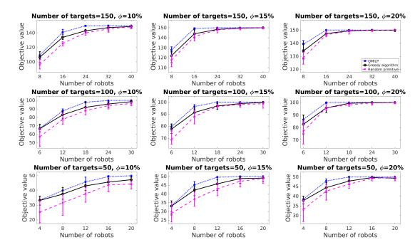
Fig. 6 Showing the comparative results of QMILP, greedy algorithm, and randomly choosing a motion primitive for WINNERTAKESALL. To generate the graphs, we varied number of robots, total number of targets, and  $\phi(\mathcal{G}_S)$ . We ran 100 trials for each case.
