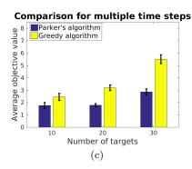
Fig. 17 Comparison with the Parker's algorithm [2]. (a) 200 instances were run. (b) 200 time steps were run. (c) 200 time steps were run to compare the metric proposed by Parker [2]. We used 10 robots for all cases. We ran 10 trials for (b) and (c). Bar graphs show the mean and standard deviation for different number of targets (10, 20 and 30 targets).
