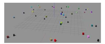
Fig. 9 Gazebo simulator showing ten robots tracking thirty randomly moving targets. We set the sensing and communication ranges to 5m and 10m, respectively.
