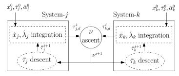
Fig. 7 This figure shows how information propagates between the two subsystems (puppets) in order to solve the networked timing problem. The initial values for system j are denoted  $\bar{\tau}_j^0$ ,  $\bar{\alpha}_j^0$  and similarly for system k.
