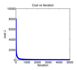
Fig. 6 Convergence of  $\cot J$  (tracking error) after performing steepest descent with Armijo step size on parameters and switching times for tracking a multi-agent drumline-inspired dance.
