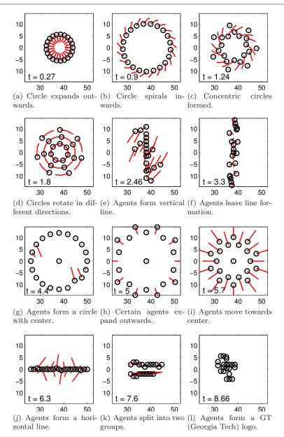
Fig. 1 Example of a complex drumline-inspired multi-agent dance, where agents switch through a sequence of controllers that were each designed for a specific maneuver. The locations of the agents are marked by O's and the lines indicate their trajectory during the past 0.3 seconds.
