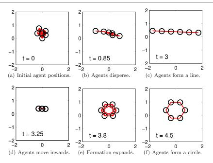
Fig. 5 Simulation of agents executing the decentralized controller sequence scripted using the locally executable  $GPS_2$ , as given in (29), for N = 6 and  $\delta = 1$ . The location of the agents are marked by O's and the lines indicate edges in the induced graph.
