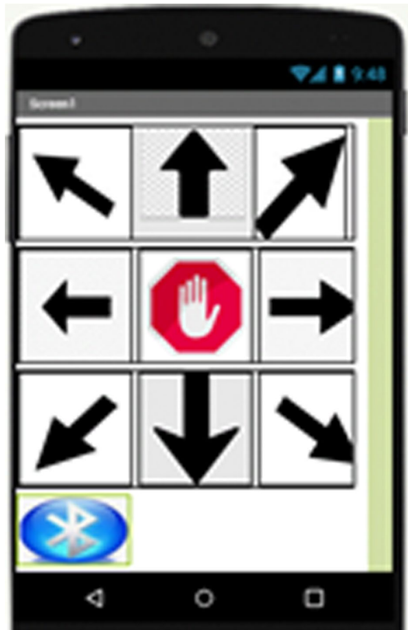
Fig. 3 Example of the AppInventor application that T2-EP1 students made to get the robot to the Chorinho (Grossi, 2006) rhythm. The connection to the robot was through Bluetooth. Source: Author's photo library
