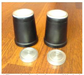
Fig. 1 Electret ion chamber detectors (200 ml volume)
