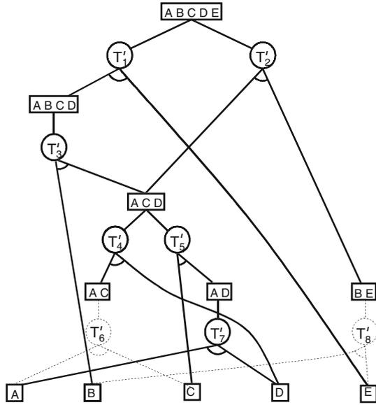
**Fig. 2** The simplified disassembly *And/Or* graph for the system ABCDE when substituting part D
