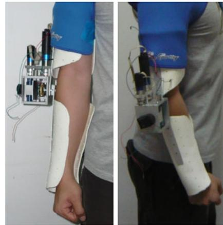
Fig. 9 CCEA exoskeleton for a human elbow
