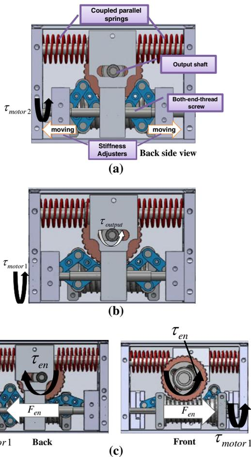
**Fig. 5** Stiffness adjustment process and continuous-state coupled elastic actuation mechanism. **a** Motor 2 drives the stiffness adjusters that carry a pair of four-bar linkage. **b** Motor 1 drives the output shaft via a worm and gear pair. Output torque will be generated only when there is environment torque on the output link. **c** Load torque on the output shaft moves the worm, and shortens one hand side springs and lengthens the other hand side springs
