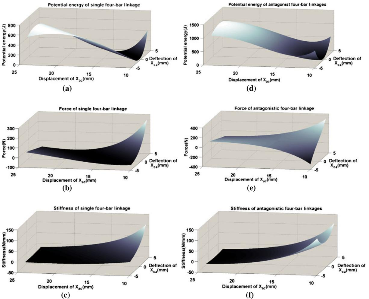
**Fig. 8** Properties of the designed CCEA system. **a** Potential energy of single four-bar linkage. **b** Force of single four-bar linkage. **c** Stiffness of single four-bar linkage. **d**
