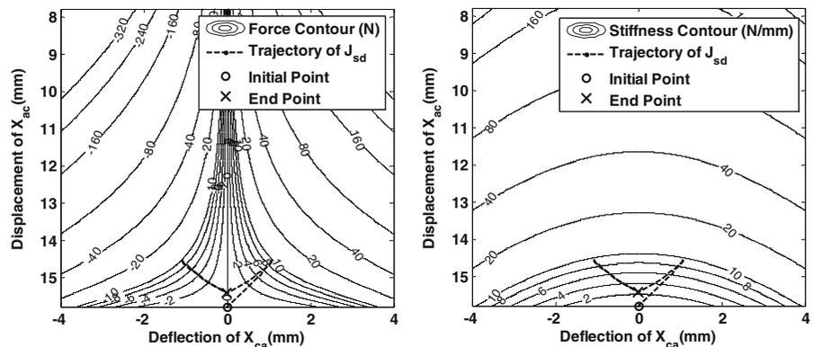
**Fig. 14** Experimental results for the force and stiffness control in the CCEA
