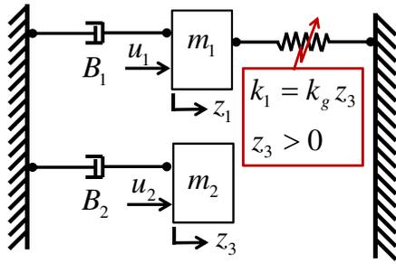
**Q4** Fig. 6 The CCEA can be modeled as this simplified model with two motors. The mass, damper, and force of Motor 1 are  $m_1$ ,  $B_1$ , and  $u_1$ . The mass, damper, and force of Motor 2 are  $m_2$ ,  $B_2$ , and  $u_2$ . The displacements of Motor 1 and Motor 2 are  $z_1$  and  $z_2$ . The stiffness of the spring in the four-bar linkage is  $k_g$ . Motor 1 is used to actuate the output link, and Motor 2 is used to change the stiffness ( $k_1$ ) of the CCEA
