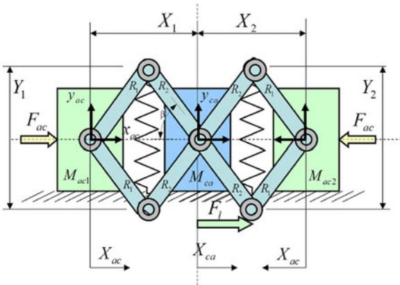
**Fig. 3** Topology of the antagonistic coupled elastic actuation
