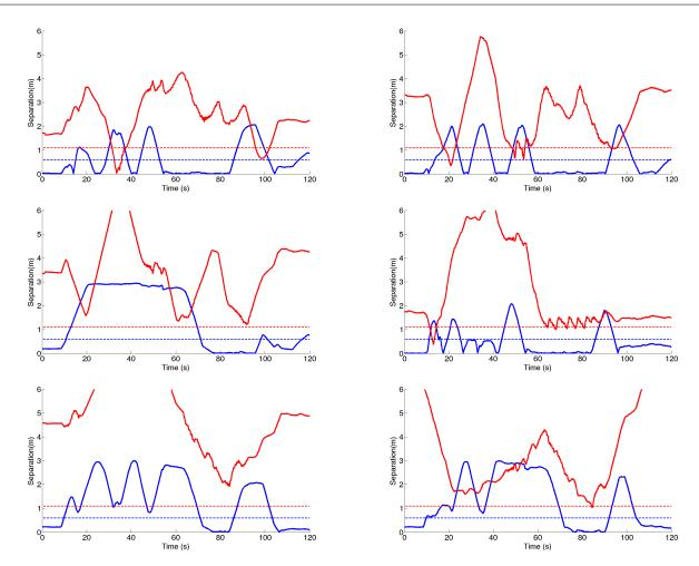
Fig. 13 Horizontal (red line) and vertical (blue line) separation between quadrotors during Experiment III. The minimum separation distances are shown in dashed line. These plots, from left to right and top to bottom represent the separations of quadrotors Q1-Q2, Q1-Q3, Q1-Q4, Q2-Q3, Q2-Q4, Q3-Q4.
