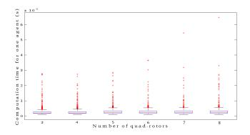
Fig. 6 Distribution of the execution computation time in proposed algorithm for one agent with the number of vehicles in the system. The median of each distribution is indicated in red, the blue box represent the 25th and 75th percentiles and the 3rd and 97th percentiles are indicated in black. Red marks represent the outliers.
