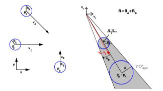
**Fig. 1** a) On the left side, a scenario involving three robots (A, B and C) on collision course is represented. b) This scenario leads to  $VO_{A|B}^{\tau}$  which is represented on the right side. The minimum reaction robots A and B have to perform in order to avoid their potential collision is represented by  $u_B$ .
