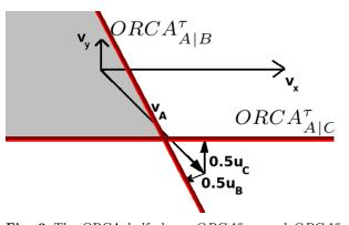
**Fig. 2** The ORCA half-planes  $ORCA_{A|B}^{\tau}$  and  $ORCA_{A|C}^{\tau}$  that robots B, C induce in robot A are represented. The region of allowed velocities robot A can take is given by the intersection of these half-planes. This region is filled in light gray.
