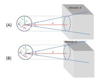
Fig. 3 Velocity obstacles induced by obstacle O to an agent in two different instants.
