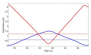
Fig. 11 Horizontal (red line) and vertical (blue line) separation between the aerial robots during Experiment II. The minimum separation distances are shown in dashed line.
