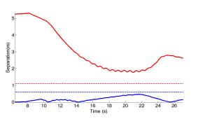
Fig. 9 Horizontal (red line) and vertical (blue line) separation between the aerial robots during Experiment 1. The minimum separation distances are shown in dashed line.
