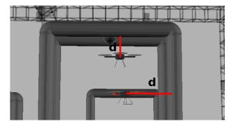
Fig. 4 Concave obstacles can break the time continuity of the distance vector. They have to be decomposed into several convex obstacles in a preprocessing step. d is the horizontal or vertical separation between a quadrotor and the closer static obstacle.
